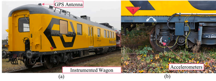
Fig. 4. The ABA measurement system instrumented on the dedicated wagon: (a) a GPS antenna (source of photo: TU Delft OpenCourseWare), (b) accelerometers attached to an axle box.
