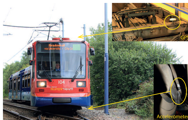
Figure 3. Axle box acceleration system used with close-ups of the GPS antenna and an accelerometer.
