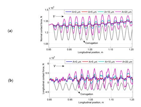
**Figure 11.** Dynamic wheel-rail contact forces obtained for the corrugation in Figure 3 with  $\theta = 0$  and P4 at 1.2 m (1.2 m is in the middle of a sleeper and 0.9 m is at the midpoint between two sleepers.). (a) Normal contact force. (b) Longitudinal contact force.
