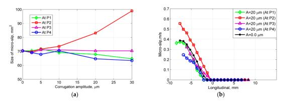
**Figure 7.** Size of the slip zone as a function of the corrugation amplitude and slip distribution along the longitudinal axis y = 0 mm at the four positions. (a) Size of slip zone; (b) slip along the longitudinal axis y = 0 mm.
