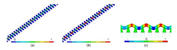
**Figure 10.** Modal analysis of the two major frequencies (1185 and 1296 Hz) shown in Figure 9: (a) rail vertical mode at 1185 Hz and (b) rail longitudinal mode at 1291 Hz, in comparison with the closest vertical pin-pin mode at 1100 Hz shown in (c).
