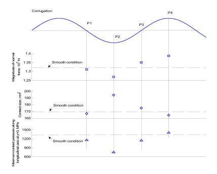
**Figure 5.** Magnitude of the normal force, contact size and maximum pressure along the longitudinal axis at (y = 0 mm) at the four analyzed positions P1, P2, P3 and P4 (A = 20  $\mu$ m).
