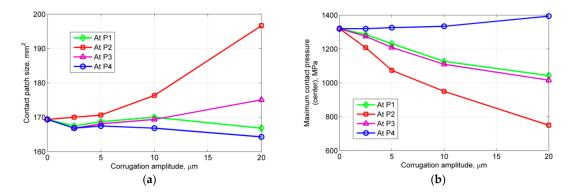
**Figure 4.** Influence of corrugation amplitude on the size of the contact patch and the maximum contact pressure along the longitudinal axis y = 0 mm. (a) Contact size; (b) contact pressure.
