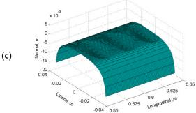
**Figure 3.** Modeled corrugation: (a) field measurement of corrugation (27–33 mm bandpass filtering); (b) schematic diagram of the corrugation and 4 positions (blue line: P1, red line: P2, green line: P3 and magenta line: P4); and (c) illustration of the applied corrugation (Corrugation 2 with P2 at 0.6 m) in the rail surface with  $5 \times$  magnification (only 3 complete waves are plotted).
