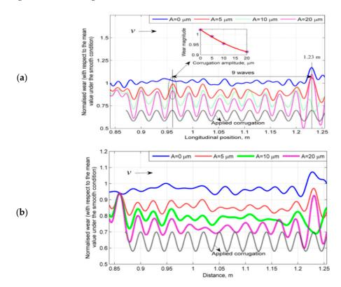
**Figure 8.** Distribution of wear at different corrugation amplitudes obtained for the corrugation in Figure 3b with  $\theta = 0$  and P4 at 1.2 m. The middle of a sleeper is at 1.2 m, and the midpoint between two sleepers is at 0.9 m. (a) High-pass filtered at  $\lambda = 20$  mm. (b) High-pass filtered at  $\lambda = 30$  mm.
