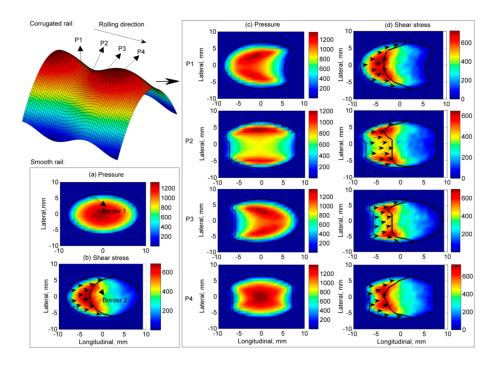
**Figure 6.** Contact pressure, shear stress, contact patch, adhesion-slip distributions and vector graphs of micro-slips (vectors in Figure  $6\mathbf{b}$ , $\mathbf{d}$ ) when  $A = 20~\mu m$  along one corrugation wavelength (P1–P4) (projection onto the xOy plane; Border 1: contact patch border; Border 2: adhesion-slip distribution border).
