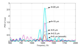
**Figure 9.** Power spectral density (PSD) of wear  $\lambda = 30$  mm, with a major peak at 1296 Hz and a secondary peak at 1185 Hz, when  $A = 20 \mu m$ .
